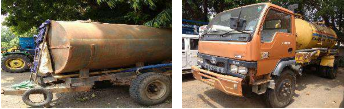
Figure 4-9: -Existing cesspool emptying vehicles with ULB
